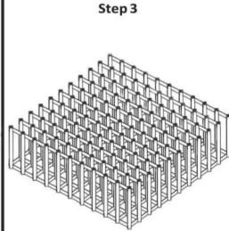
Very important! Insert one section of the metal frame only half way down into the wood pieces.
