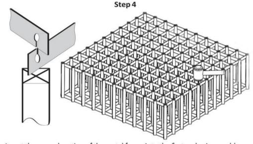
Insert the second section of the metal frame into the first and using a rubber mallet complete the installation into the wood pieces.
