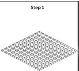
Assemble the bottom metal frame on a flat surface.
