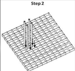
Line up and insert the wood rack pieces into the metal frame. Use a rubber mallet to install into the metal cross frame. Repeat until all wood rack pieces are installed.
