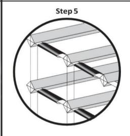
The bottle neck label protectors snap onto the front side of the metal frame as shown.
